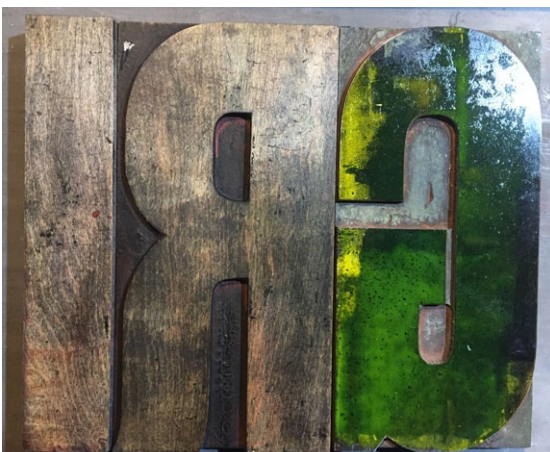
'The 'G' had ink left on it and was returned to the type case. All type should be clean and look like the 'T' and 'R' letters.
